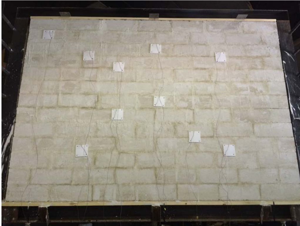
Figure 7: Unexposed side prior to the fire test.
