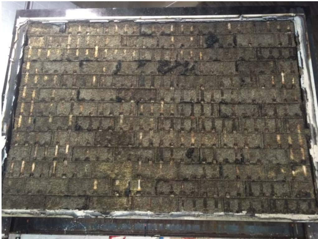
Figure 10: Exposed side after the hose stream test.
